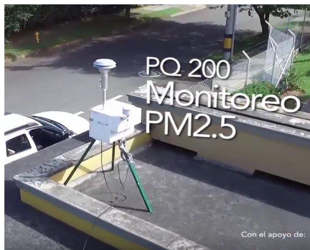
Figure 6 PQ 200 BGI Mesa Labs Ambient air particulate sampler used by SIATA
