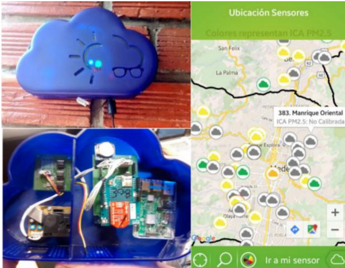
Figure 8 Low cost sensor platform and app to monitoring it
