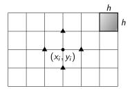
$$(\Delta u)_{v_i} = \frac{1}{h^2} \left[ u(x_{i+1}, y_i) + u(x_{i-1}, y_i) + u(x_i, y_{i-1}) + u(x_i, y_{i+1}) - 4u(x_i, y_i) \right] ,$$
