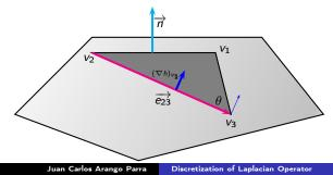
The magnitude of this vector can also be written  $\|(\nabla h)_{v_1}\| = \frac{1}{2A} \|\overrightarrow{e_{23}}\|$ where  $\mathcal{A}$  is the area of the triangular face. The gradient associated with the vertex  $v_1$  is written as
